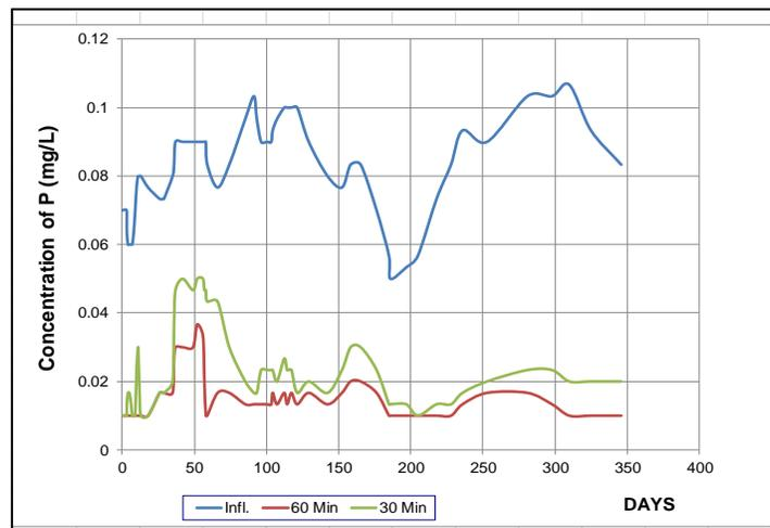
The low P levels are similar to P levels found in waterways and agricultural runoff water (0.05 to 0.12 mg/L). As can be seen, P was lowered to below 0.04 mg/L for over 220 days. Readings vary, due to measurement sensitivity in a colorimeter with a limit of  $\pm 0.02$  mg/L.
