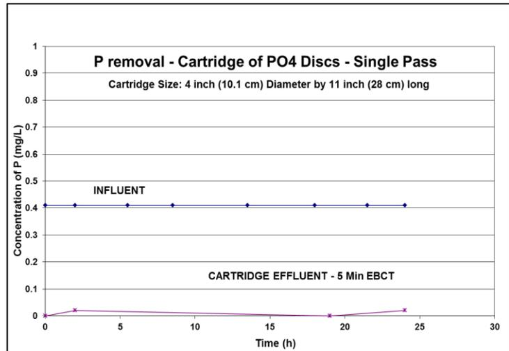
concentration remained below 0.05 mg/L. In these tests, P in the water was periodically increased to 1 mg/L and time to recovery to lower levels was determined. P was lowered to below 0.1 within a few hours and back to lower levels shown in the graph, typically within 24 hours. This simulates conditions found in some wetlands and natural swimming pools.
