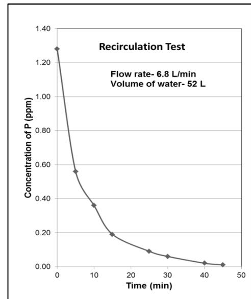
**Recycling** examples are shown where water was recycled through a a column of PO4 Sponge monoliths. P is lowered from 1.2 mg/L to below 0.1 mg/L in 25 min and to 0.01 ppm in 45 min.
